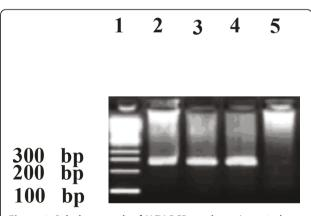
Figure 1 Gel photograph of HCV PCR products: Lane 1 shows 100 bp DNA ladder, lane 2, and 3 are the positive samples for active HCV infection showing 285 bp nested PCR product, Lane 4 is positive HCV control while Lane 5 is negative control.
