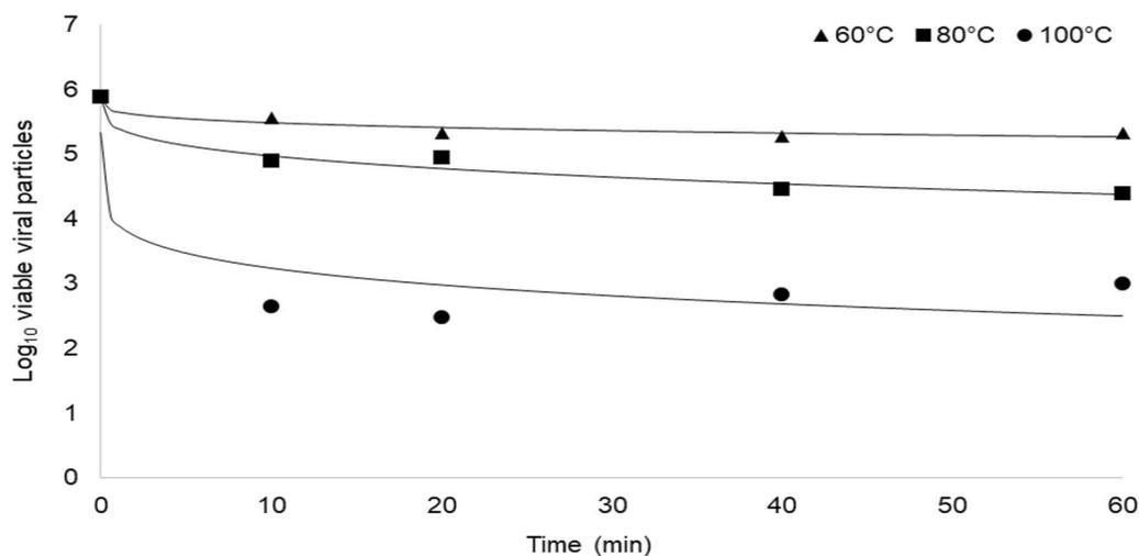
**Fig. 4** Inactivation kinetics of EhV. Temperature and time inactivation kinetics as determined from viability PCR for EhV-86 treated at 60 °C, 80 °C, and 100 °C for 10 min, 20 min, 40 min, and 60 min. A Weibull model was fitted to the data with  $R^2$  values of 0.93, 0.97 and 0.95, for the 60 °C, 80 °C, and 100 °C data sets, respectively
